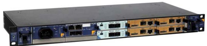
Compact TORNADO-MTCA® DSP/FPGA modular system with two T/AX-DSFPX network AMC-modules and four TORNADO-A6678® DSP/FPGA M/S AMC-modules in 19" 6-slot MicroTCA® chassis with 10GbE backplane switch
