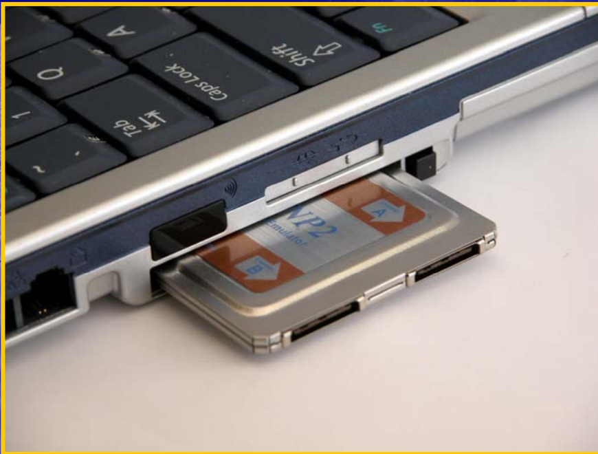
Installation into the PCMCIA PC Card (CardBus) slot of the Notebook PC
