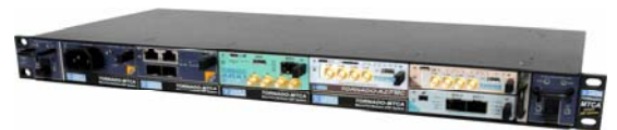
TORNADO-MTCA® DSP modular system including TORNADO-AZU+/FMC+ and TORNADO-A6678/FMC AMC modules with FMC A/D submodules, TORNADO-ARX1 RF AMC module and T AX-DSFPX AMC module with 10GbE SFP+ ports all installed into MicroTCA® 1U chassis with 10GbE switching fabric
