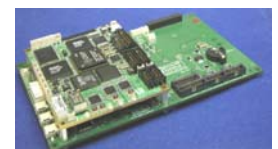
TORNADO-PX/DDC4G installed onto TORNADO-E2/6713
