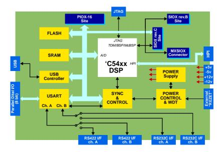
TORNADO-E54x are high performance embedded DSP controllers with the industry standard 3U form-factor for real-time data acquisition and DSP. Flexible modular construction and a variety of "off-the-shelf" AD/DA/DIO and I/O coprocessor expansion daughter card modules make TORNADO-E54x an ideal selection for embedded telecommunication, telephony, multimedia, instrumentation, digital radio and many more application.
