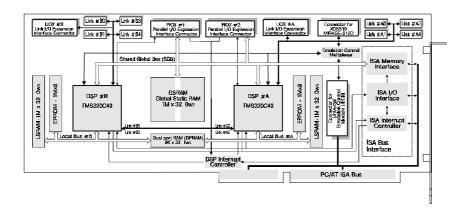
*TORNADO-40D* is a powerful, high performance and flexible multiprocessor DSP platform for real-time signal acquisition, floating-point DSP and TMS320 DSP systems development and dignostics.
