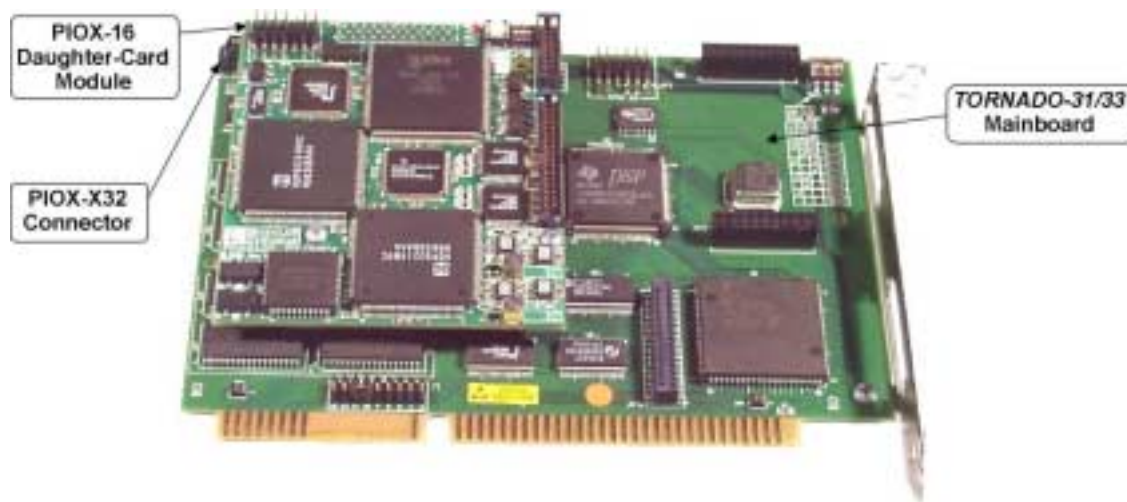
Fig.2-6b. Installation of PIOX-16 DCM onto TORNADO-31/33 mainboard.
