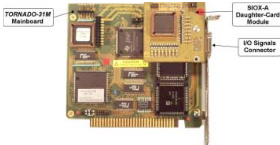
Fig.2-12e. TORNADO-31M mainboard with SIOX DCM for installation into standard desktop PC chassis.
