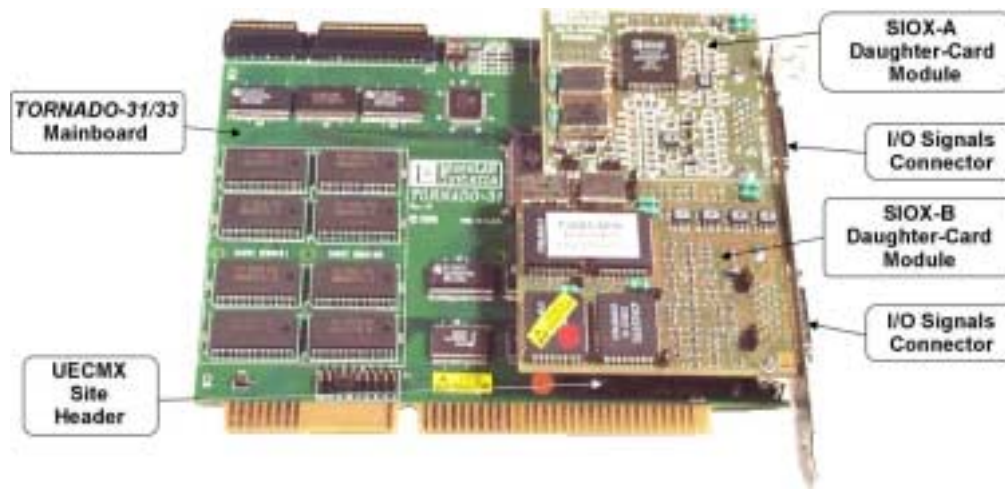
Fig.2-12a. TORNADO-31/33 mainboard with SIOX-A and SIOX-B DCMs.
