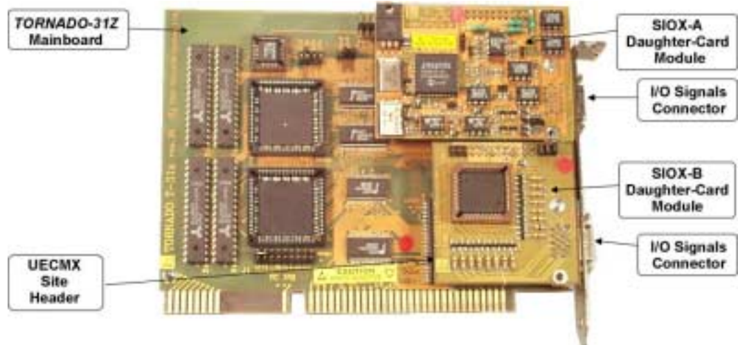
Fig.2-12c. TORNADO-31Z mainboard with SIOX-A and SIOX-B DCMs.
