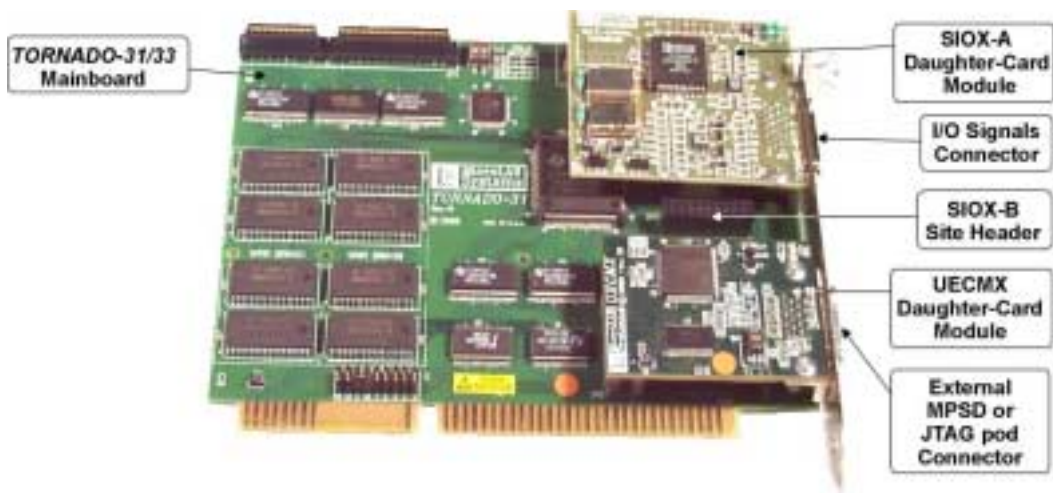
Fig.2-12b. TORNADO-31/33 mainboard with SIOX-A and UECMX DCMs..
