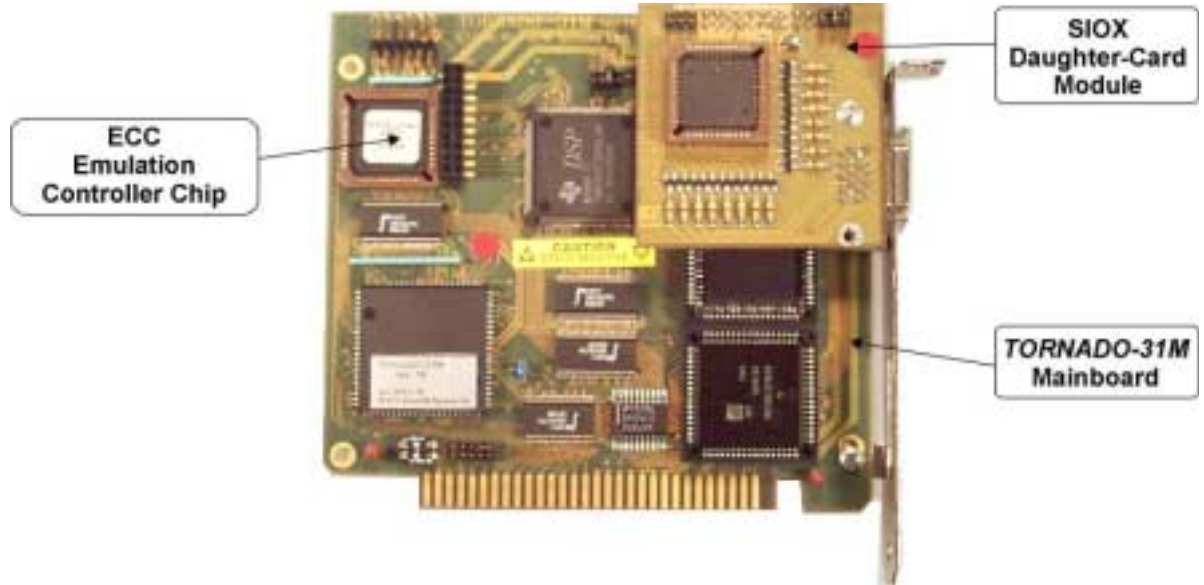
Fig.1-1c. TORNADO-31M DSP system with SIOX DCM and ECC emulation controller.
