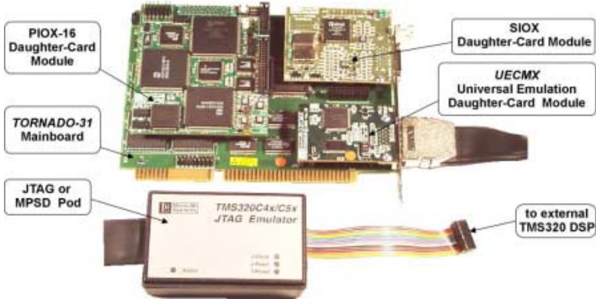
Fig.1-1a. TORNADO-31 DSP system with SIOX and PIOX-16 DCM, UECMX emulator DCM and external JTAG pod.
