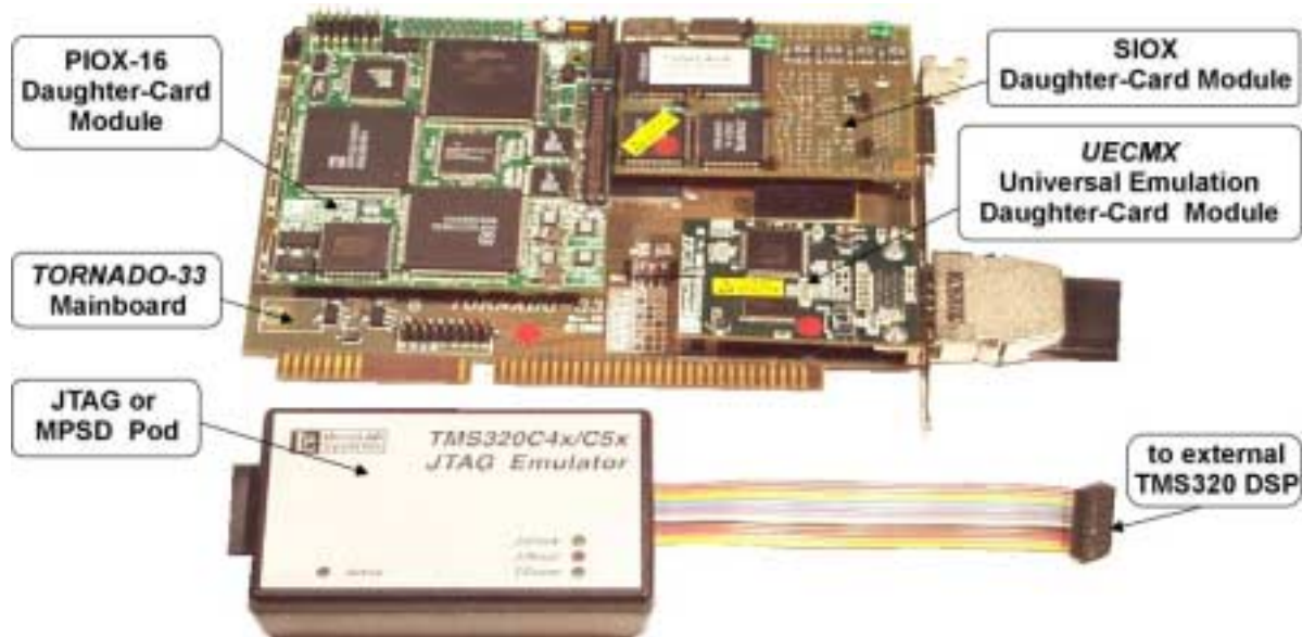
Fig.1-1d. TORNADO-33 DSP system with SIOX and PIOX-16 DCM, UECMX emulator DCM and external JTAG pod.
