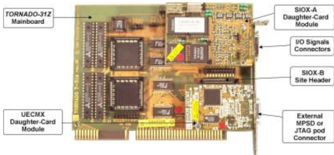
Fig.2-12d. TORNADO-31Z mainboard with SIOX-A and UECMX DCMs..
