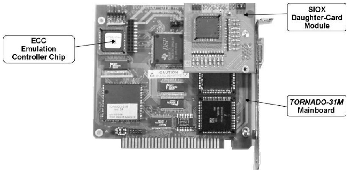
Fig.1-1c. TORNADO-31M DSP system board with SIOX daughter-card module and ECC emulation controller.
