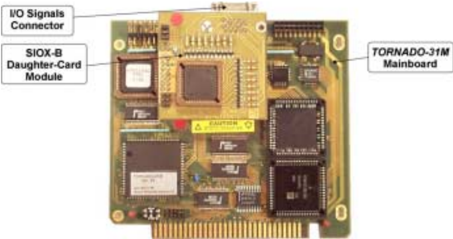
Fig.2-12f. TORNADO-31M mainboard with SIOX DCM for installation into industrial MicroPC™ chassis.
