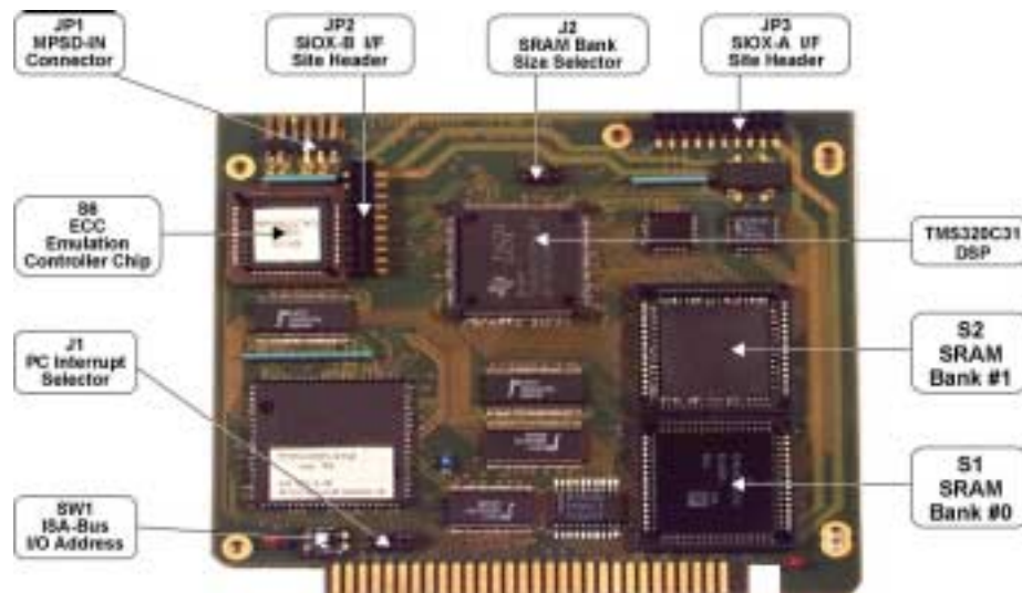
Fig.2-2c. Construction of TORNADO-31M mainboard.
