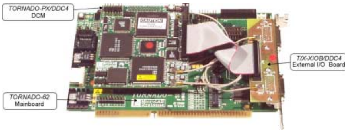
Fig. 1-4. TORNADO-PX/DDC4 DCM with T/X-XIOB/DDC4 external I/O board installed onto TORNADO-62 PC plug-in DSP system.
