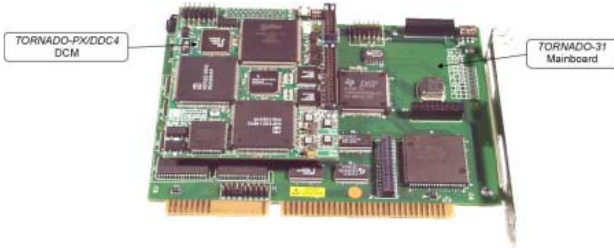
Fig. 1-2. TORNADO-PX/DDC4 DCM installed onto TORNADO-31 mainboard.
