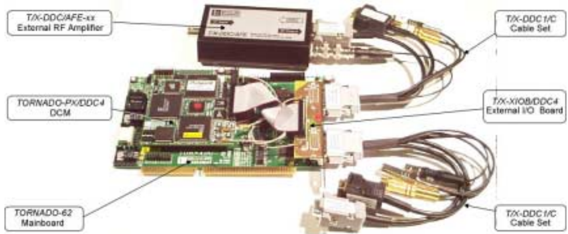
Fig. 1-5. TORNADO-62 PC plug-in DSP system with TORNADO-PX/DDC4 DCM, T/X-XIOB/DDC4 external I/O board, T/X-DDC1/C external I/O cable set and T/X-DDC/AFE-xx external RF amplifier.
