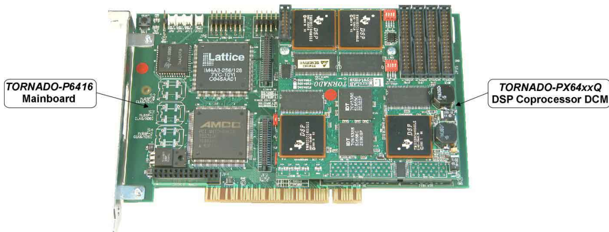
Fig. 1-2a. TORNADO-PX64xxQ DCM installed into 32-bit PIOX-32 DCM site of host TORNADO-P6416 PCI-bus plug-in DSP system.
