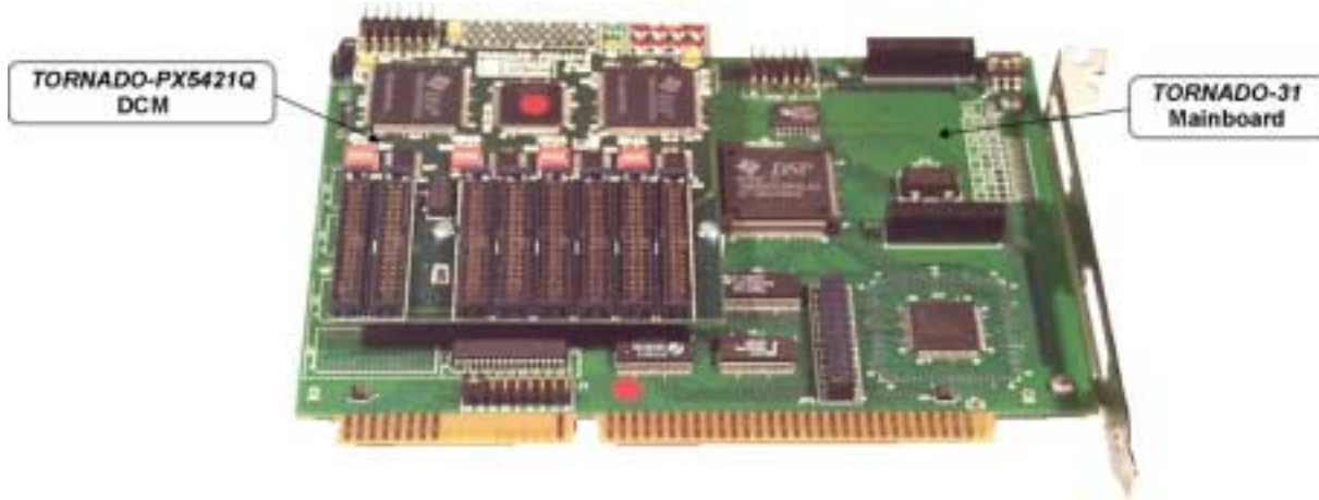
Fig. 1-2. TORNADO-PX5421Q DCM installed onto TORNADO-31 DSP system.
