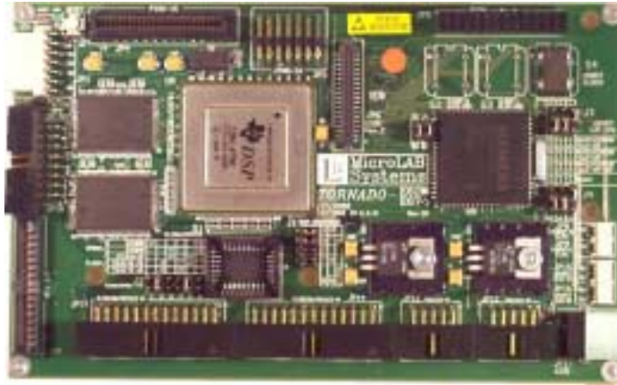
Fig.1-1a. TORNADO-E62/E67 DSP controllers board.
