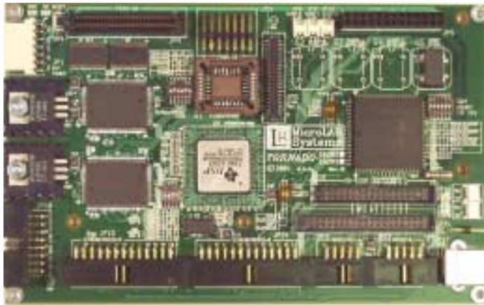
Fig.1-1b. TORNADO-E6202/E6203 DSP controllers board.
