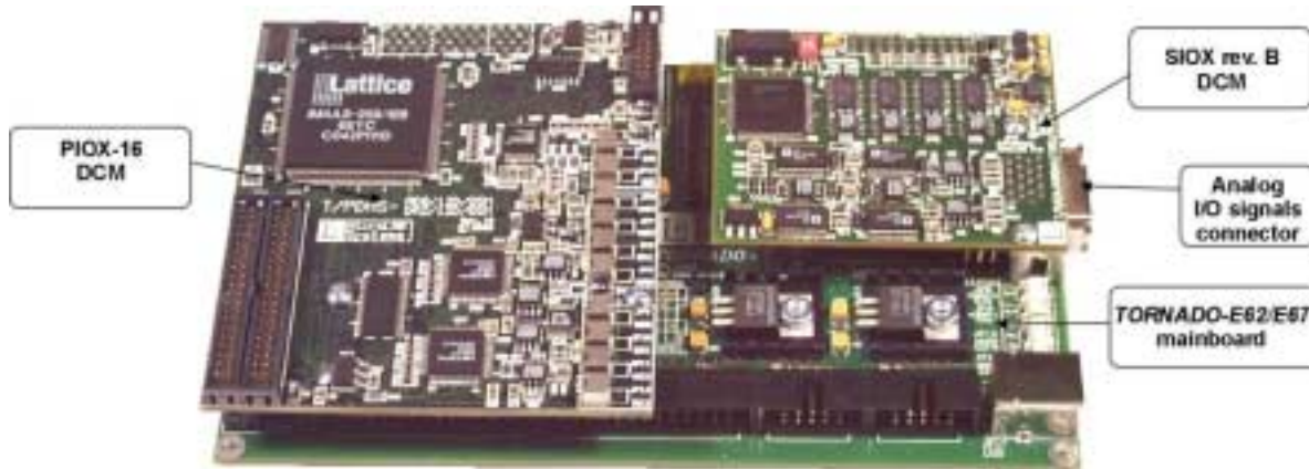
Fig.1-2a. TORNADO-E62/E67 DSP controller with SIOX rev.B and PIOX-16 DCM installed.
