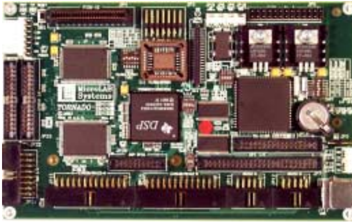
Fig.1-1c. TORNADO-E6414/E6415/E6416 DSP controllers board.
