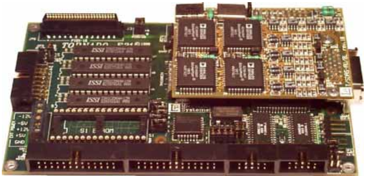
Fig.1-1. TORNADO-E31 DSP controller board with SIOX daughter card module.
