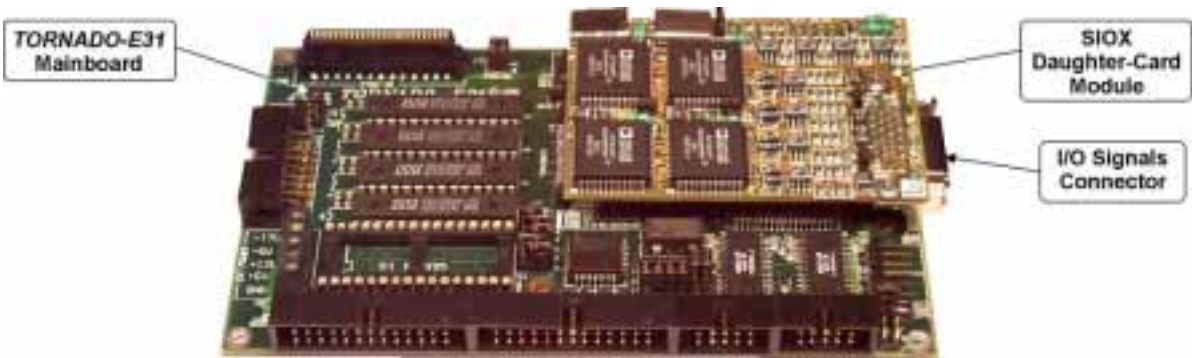
Fig.2-7. TORNADO-E31 with SIOX daughter-card module installed.
