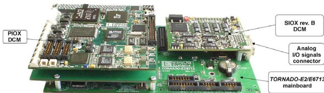
Figure 1-3. TORNADO-E2/6713 DSP controller with SIOX rev.B and PIOX DCM installed.
