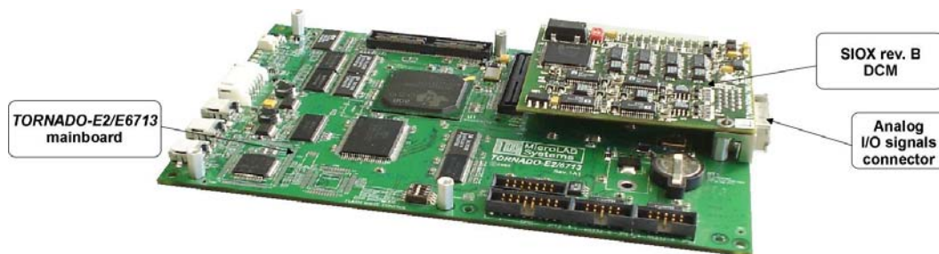
Figure C-1. TORNADO-E2/6713 board with SIOX rev.B DCM installed.
