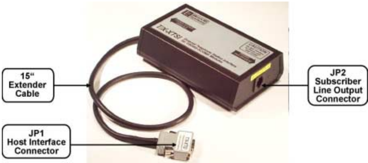
Fig. A-1. Connectors layout for T/X-XTSI external telephone station interface.
