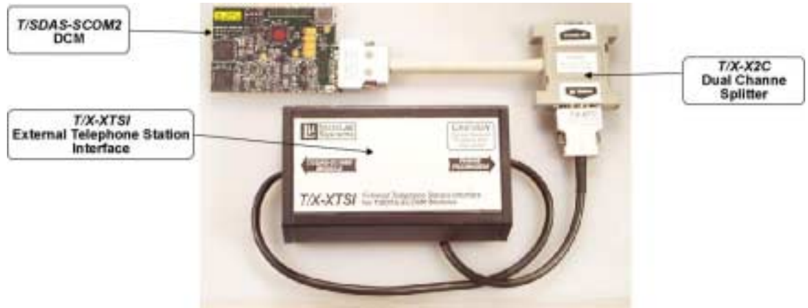
Fig. 1-3. T/SDAS-SCOM2 DCM with external dual-channel splitter (T/X-X2C) and one external T/X-XTSI external telephone station interface.
