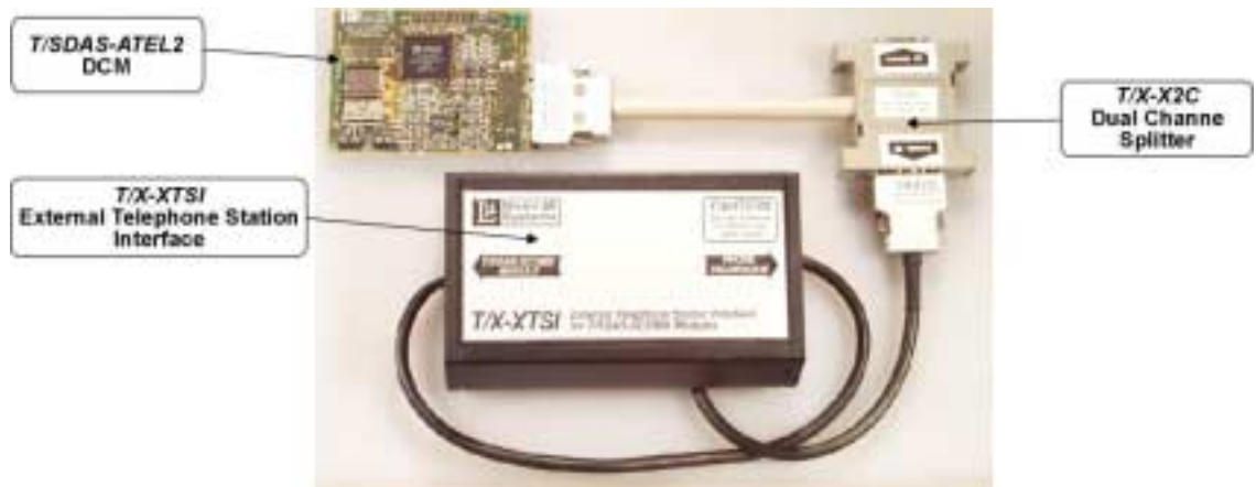
Fig. 1-4. T/SDAS-ATEL2 DCM with external dual-channel splitter (T/X-X2C) and one external T/X-XTSI external telephone station interface.
