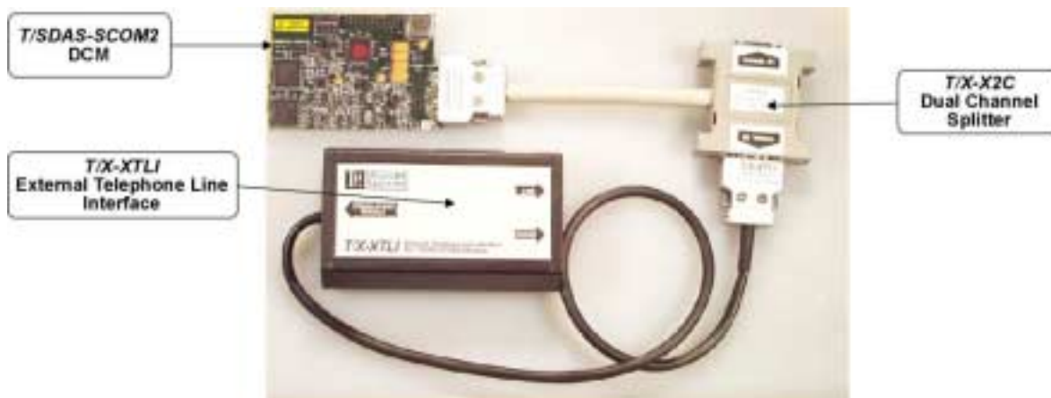
Fig. 1-3. T/SDAS-SCOM2 DCM with external dual-channel splitter ( T/X-X2C ) and one external T/X-XTLI external telephone line interface.
