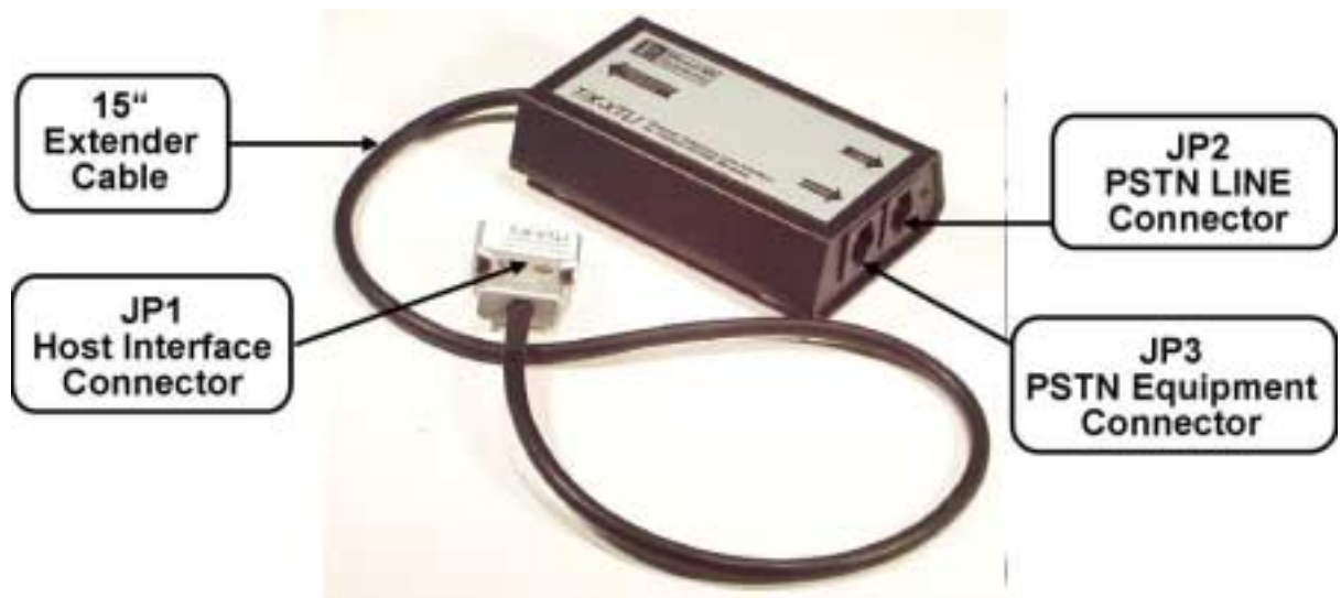
Fig. A-1. Connectors layout for T/X-XTLI external telephone line interface.
