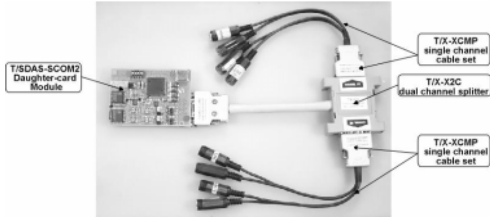
Fig. 1-6. T/SDAS-SCOM2 daughter-card module with T/X-X2C dual-channel splitter and two T/X-XCMP single-channel cable sets.
