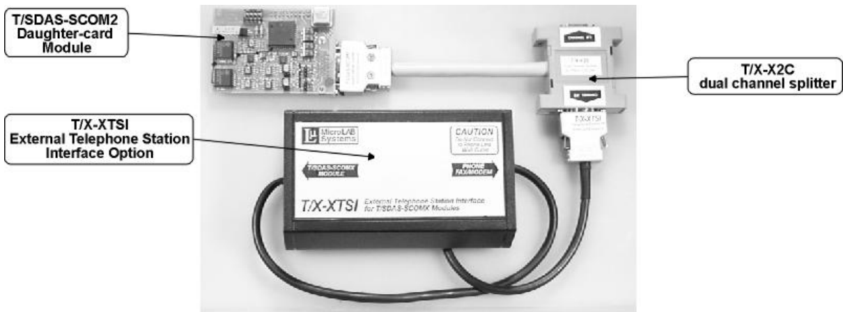
Fig. 1-8. T/SDAS-SCOM2 daughter-card module with external dual-channel splitter (T/X-X2C) and one external T/X-XTSI external telephone station interface option.
