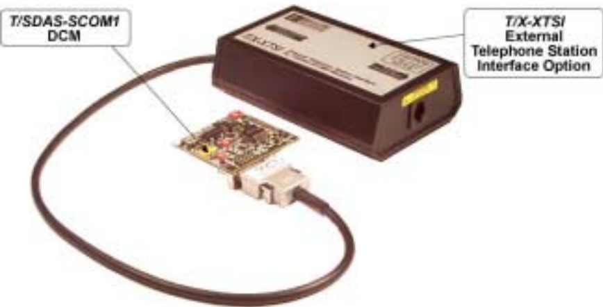
Fig. 1-5. T/SDAS-SCOM1 DCM with external T/X-XTSI external telephone station interface option.
