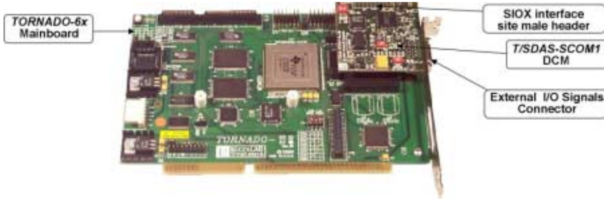
Fig. 1-2. T/SDAS-SCOM1 DCM installed onto TORNADO-62 mainboard.
