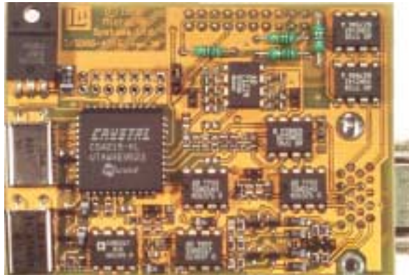
Fig. 1-1a. T/SDAS-4215 Stereo Audio SIOX DCM with Professional/Consumer I/O.
