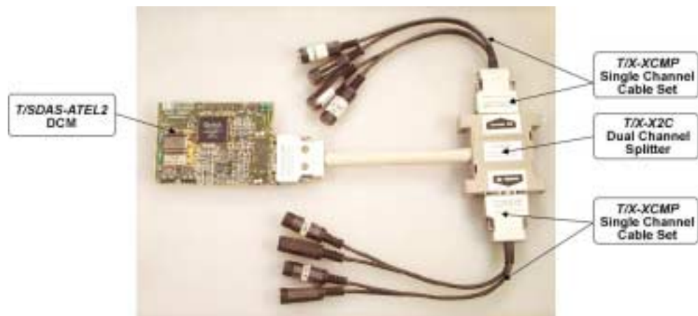
Fig. 1-9. T/SDAS-ATEL2 DCM with T/X-X2C dual-channel splitter and two T/X-XCMP single-channel cable sets.
