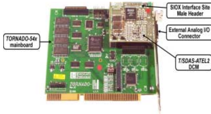
Fig. 1-2. T/SDAS-ATEL2 DCM installed onto TORNADO-54x mainboard.
