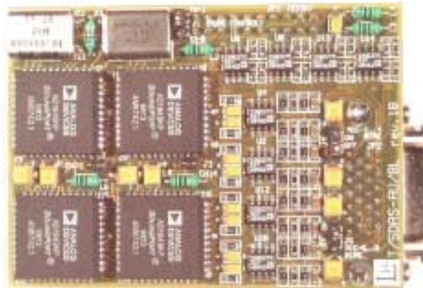
Fig. 1-1c. T/SDAS-AU/8L 8-chanel Audio SIOX DCM.
