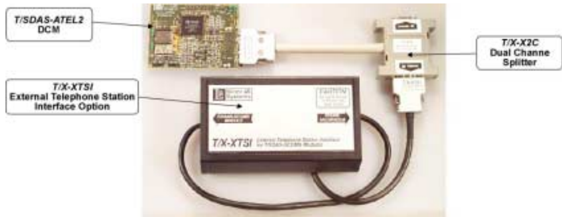
Fig. 1-11. T/SDAS-ATEL2 DCM with external dual-channel splitter (T/X-X2C) and one external T/X-XTSI external telephone station interface option.
