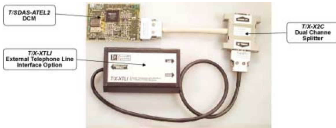
Fig. 1-10. T/SDAS-ATEL2 DCM with external dual-channel splitter ( T/X-X2C ) and one external T/X-XTLI external telephone line interface option.
