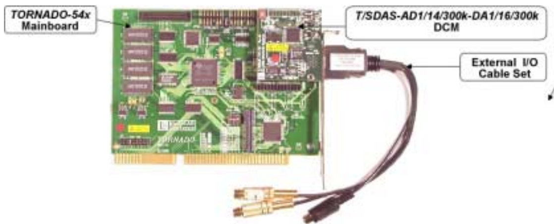
Fig. 1-2. T/SDAS-AD1/14/300K-DA1/16/300K DCM installed onto TORNADO-54x mainboard with external I/O cable set.
