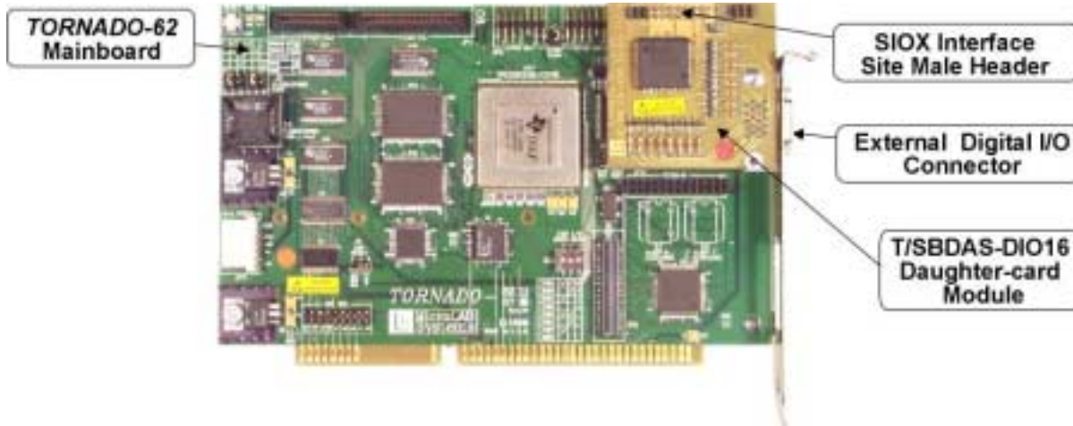
Fig. 1-2. T/SBDIO-16 DCM installed onto TORNADO-6x mainboard.
