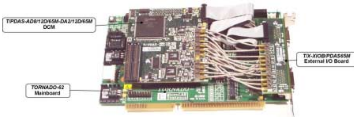
Fig. 1-4. T/PDAS-AD8/12D/65M-DA2/12D/65M DCM with T/X-XIOB/PDAS65M external I/O board installed onto TORNADO-62 PC plug-in DSP system.
