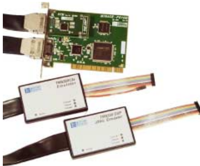
Fig.1-1. MIRAGE-P510D dual-channel emulator with MP510D/ECM emulator expansion daughter-card module and MPSD and JTAG pods.
