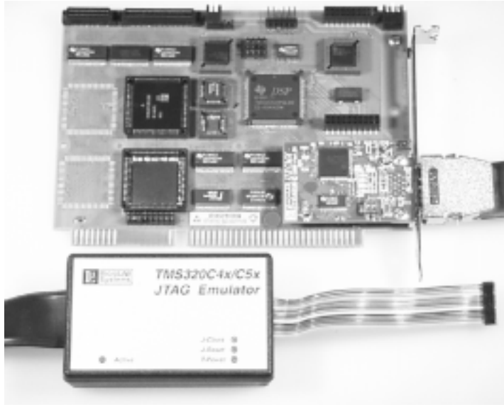
Fig.1-2. TORNADO-31 DSP system with UECMX module and optional pod.
